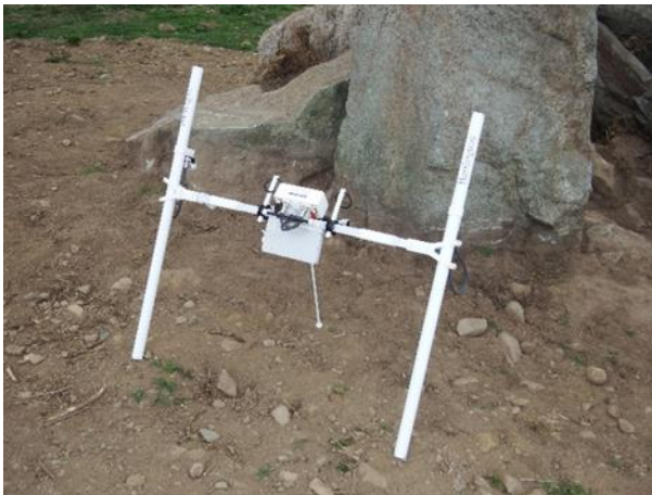
Bartington Grad 601-single axis dual sensor gradiometer.
