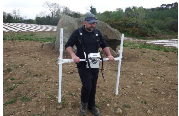
Bartington Grad 601-single axis dual sensor gradiometer.
